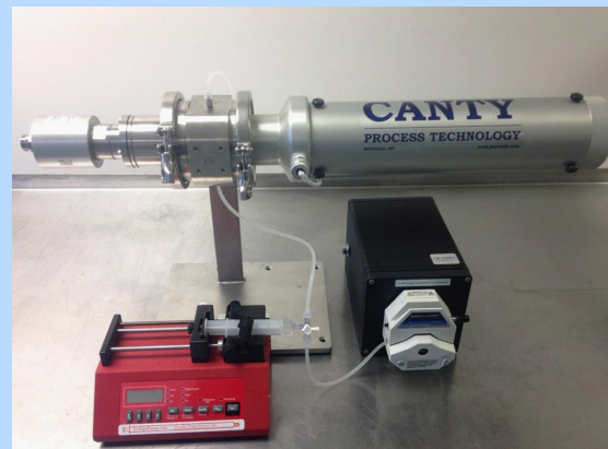
Automated syringe pump feed mechanism & dilution pump
