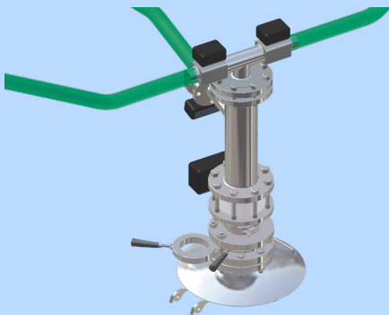
Vessel Charging with DEC PTS System
