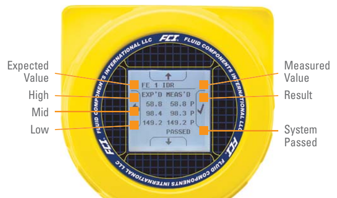
Figure 1. Front panel; all three check points show "P" (pass) and entire self-check "PASSED"
